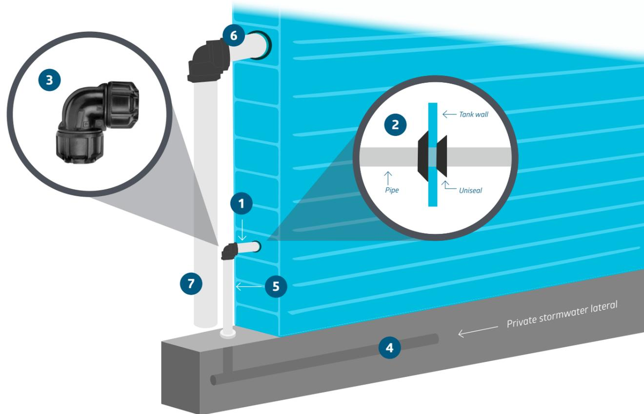
1. A short 20mm diameter pipe is inserted into the tank end at the required height (see Table 2). The pipe is held secure to the tank using a Uniseal or similar product. For a 20mm diameter pipe it is recommended to use a 31.7mm holesaw size to drill your outlet.
