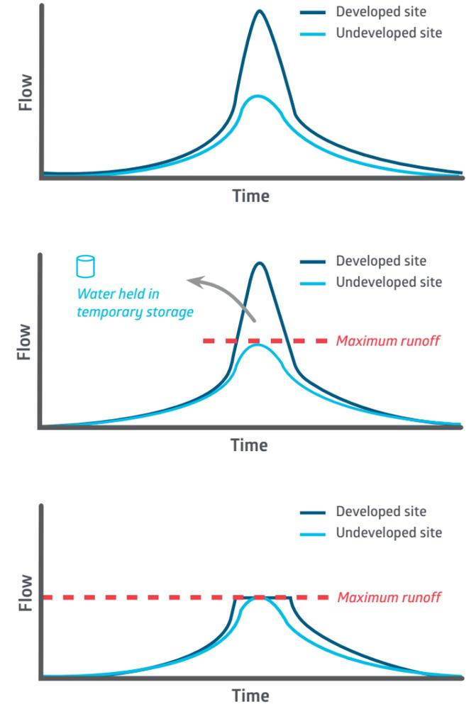
We define hydraulic neutrality as capturing post-development peak runoff so that it does not exceed the pre-development peak flow rate.
